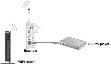
The device connects to the extender. Now the device can access your existing WiFi network through the extender.
